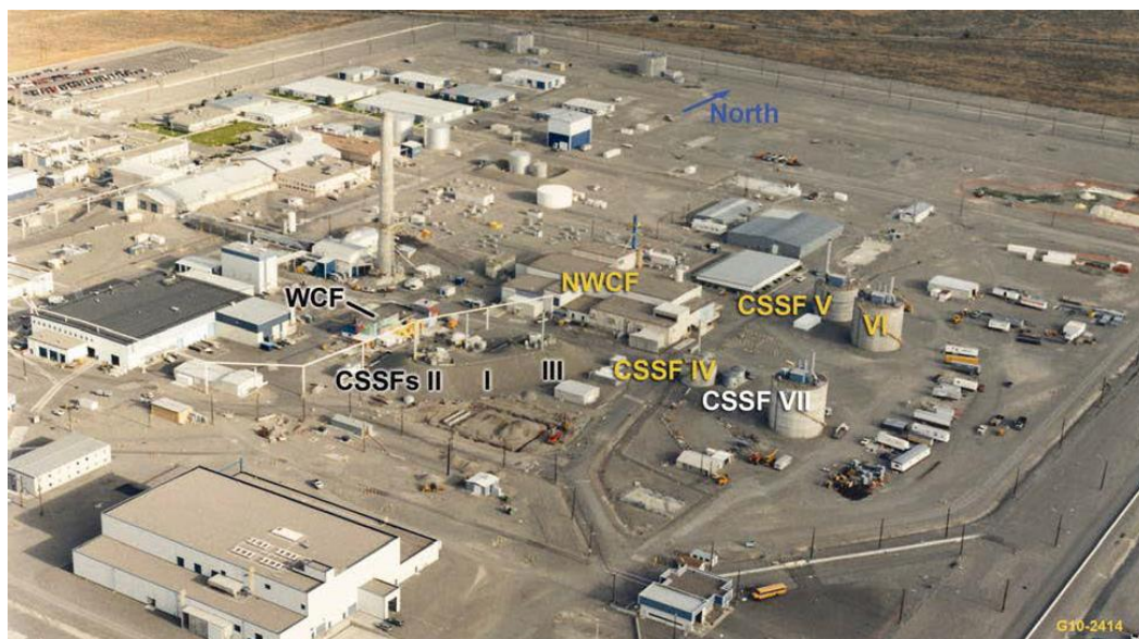
Figure 1. Aerial Photograph Showing the Waste Calcining Facility (WCF), the New Waste Calcining Facility (NWCF) now closed, and the Calcined Solids Storage Facilities (CSSFs) at the Idaho National Laboratory. DOE photo.
